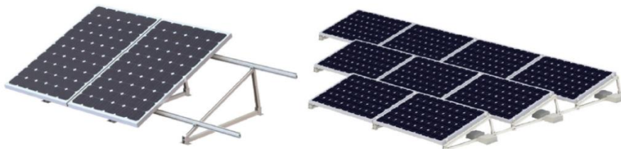
Figure 2.4- Portrait vs Landscape disposition of the solar panels. Source: Conermex
